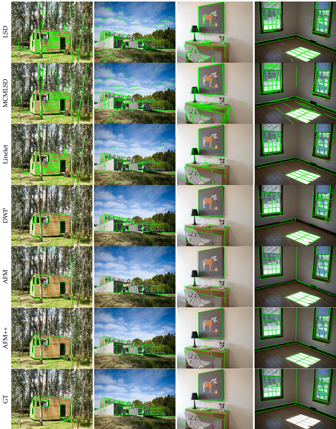
Fig. 7. Some results of line segment detection of different approaches on the Wireframe [12] dataset. From top to bottom: LSD [2], MCMLSD [3], Linelet [18], DWP [12], AFM [33] with the a-trous Residual U-Net and AFM++ proposed in this paper.
